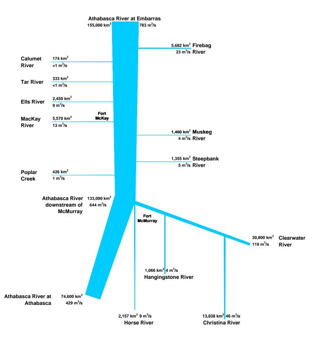
Figure 1.2 Hydrologic schematic of RAMP Focus Study Area.
